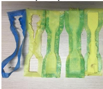
Figure (2.8) Some Failure Samples
